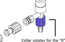
Collar rotates for the "R" type and is fixed for the standard type.
